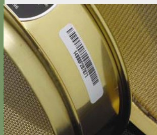
Sieve is serialized for accurate identification in your quality assurance system.
