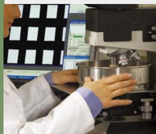
State-of-the-art image analyzer used to inspect openings and wire diameters.
